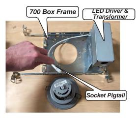
1. Install Recessed *CLARTÉ 700* Box Frame by Inserting two hanger bars into wood framing or T-Bar drop down ceiling.
