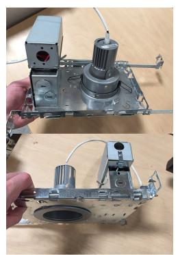
3. Plug pigtail to back of fixture and adjust fixture to desired angle.
