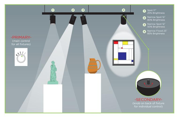
Clarté Lighting LED track fixtures will dim on the primary side of the circuit utilizing simple 2 wire forward phase magnetic low voltage dimming and/or the secondary side of the circuit for individually adjusting light levels per fixture manually bypassing the primary side dimming light level adjustment.
