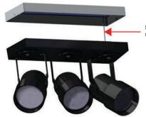
4. Align mounting plate to ballast housing.
