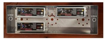
Three drivers inside housing. 1 screw on each side to secure lid.
