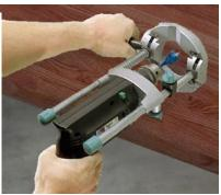
1. Use an adjustable drill holder guide and set it to 35°. From the back of the panel of wood, use a boring attachment and drill a 1" hole downward into the wood.
