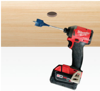
1. Drill a 13/16" hole into the ceiling.
