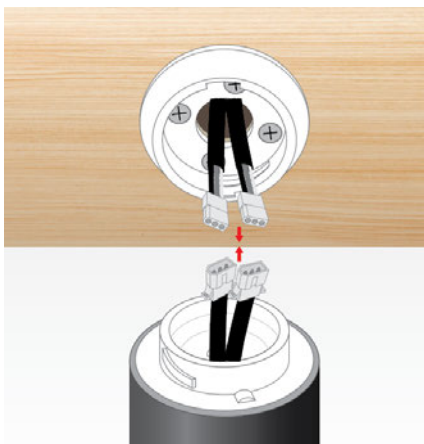
4. Connect wires from ceiling to fixture.
