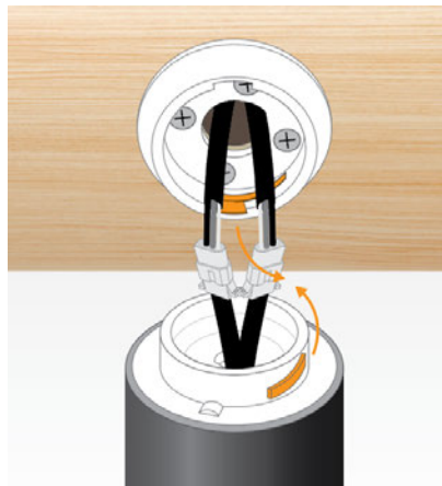
5. Line up slots (shown here in orange) then slide in and turn counter-clockwise to lock fixture in place.
