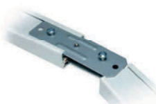
Track Reinforcement Plate Used to strengthen mechanical connection between track sections when a linear coupler is utilized. 760-GEA 21
