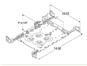
IC: Architectural Housing - Trimless, Level Plane or 1/2" Recessed.
